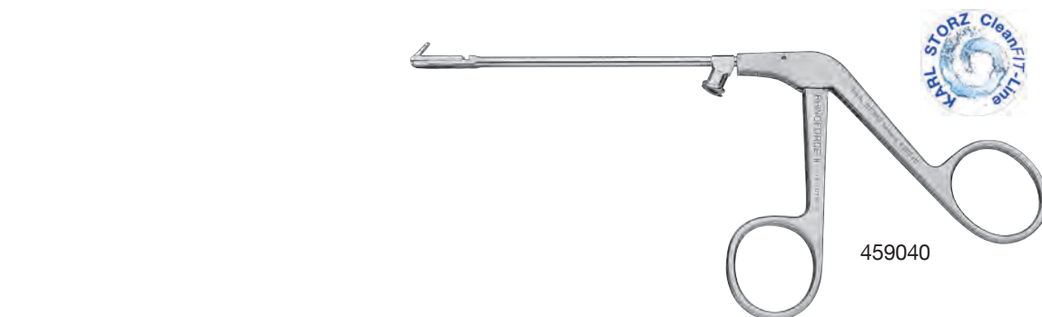
459040 PARSONS RHINOFORCE® II Punch , for partial resection of the uncinate process, upside backward cutting, movable jaw with round tip, diameter 2.5 mm, with cleaning connector, working length 10 cm
